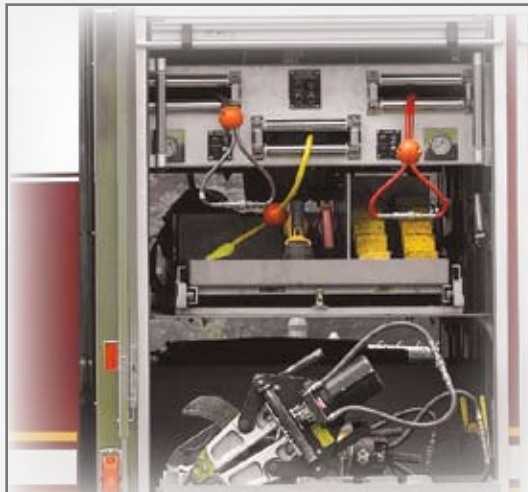
Hydraulic system compartments. Reels (roof-mounted and in rooftop compartments) and tools all in one place.
